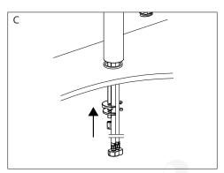
C. Attach the mounting rod to the faucet. Insert the rubber washer, metal washer, and secure the faucet with the locking nut.
