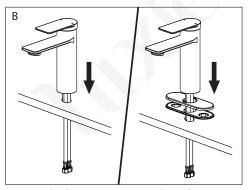
B. Attach the mounting rod to the bottom of the faucet. For single hole installation, insert the faucet through the mounting hole directly OR use the included deck plate to covert a 4 inch centerset hole pattern to a single hole pattern.
